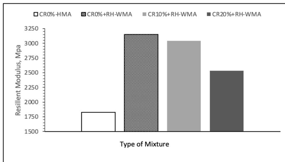
**Figure 2.** Resilient modulus of CR mixtures
