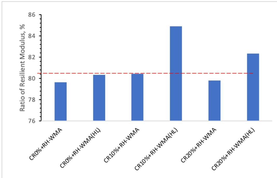
Figure 4. Effects of CR addition on moisture susceptibility
