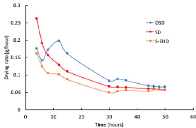
**Figure 4.** Drying rate of coffee beans against time.
