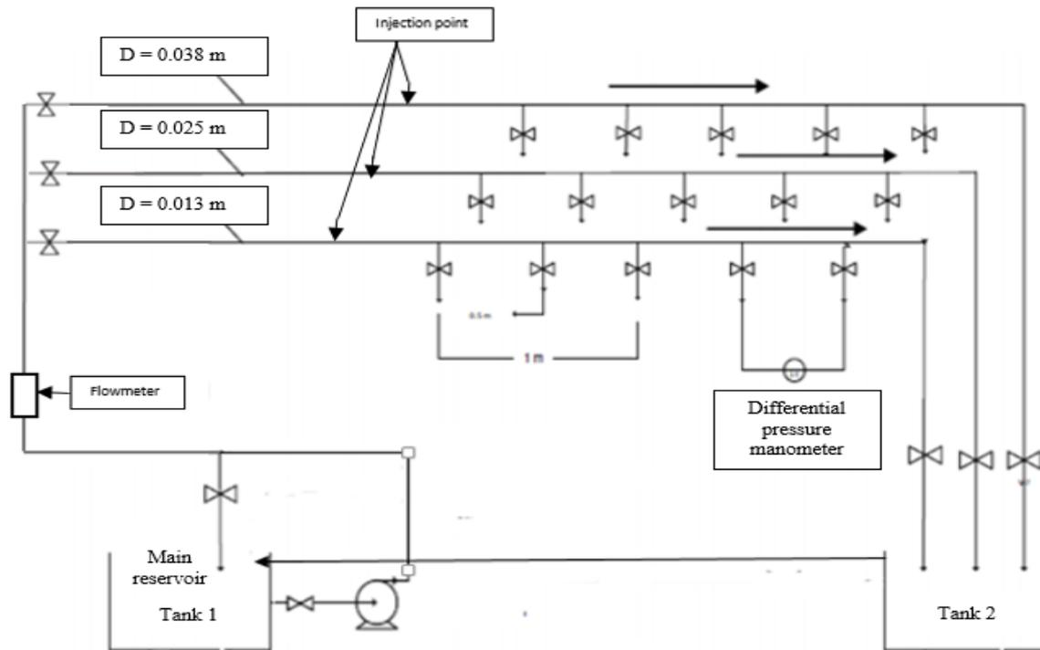
**Figure 1.** Schematic diagram of the experimental rig.
