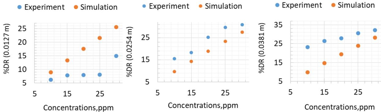
**Figure 3.** Comparison of DR obtained through experiment and simulation in individual pipe.
