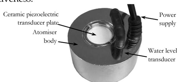
Figure 3. A commercial ultrasonic atomiser.
