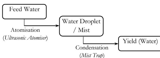
Figure 2. Ultrasonic atomisation system process flow.
