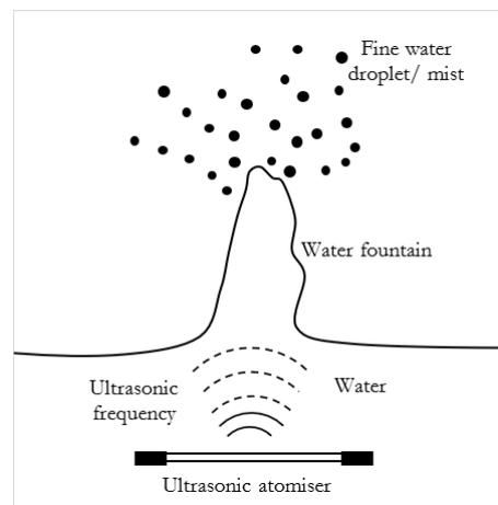
Figure 1. Water atomisation through an ultrasonic atomiser.
