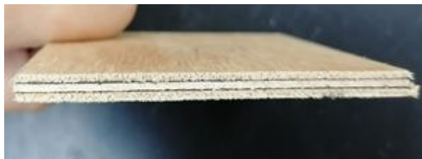
Figure 1. Sample of Laran 3-ply plywood.
