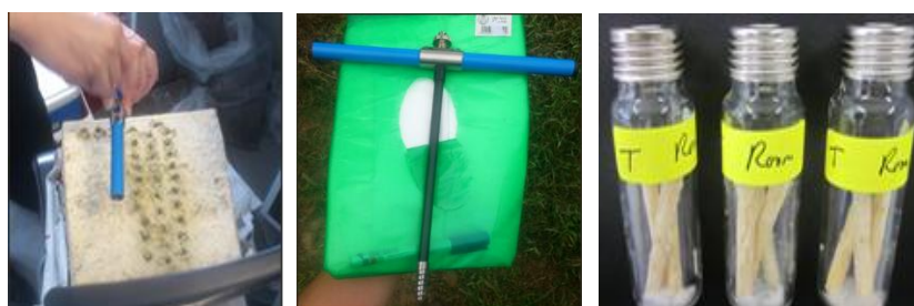
Figure 1. Trunk cores were removed from a chunk of healthy mature oil palm trunk (left) via an increment borer (middle), which were then placed into GC vials with or without G. boninense inoculum (right, inoculated vials shown).
