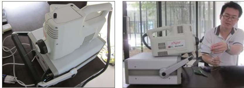
Figure 2. zNOSE™ equipment (left) and the method of reading the headspace VOCs (right).
