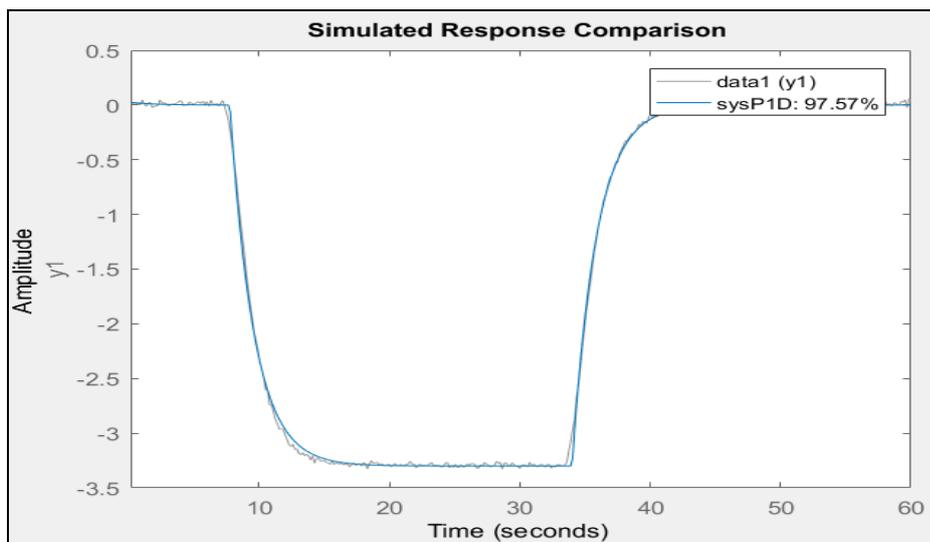
Figure 3. Predicted sysP1D versus real time data (y1).
