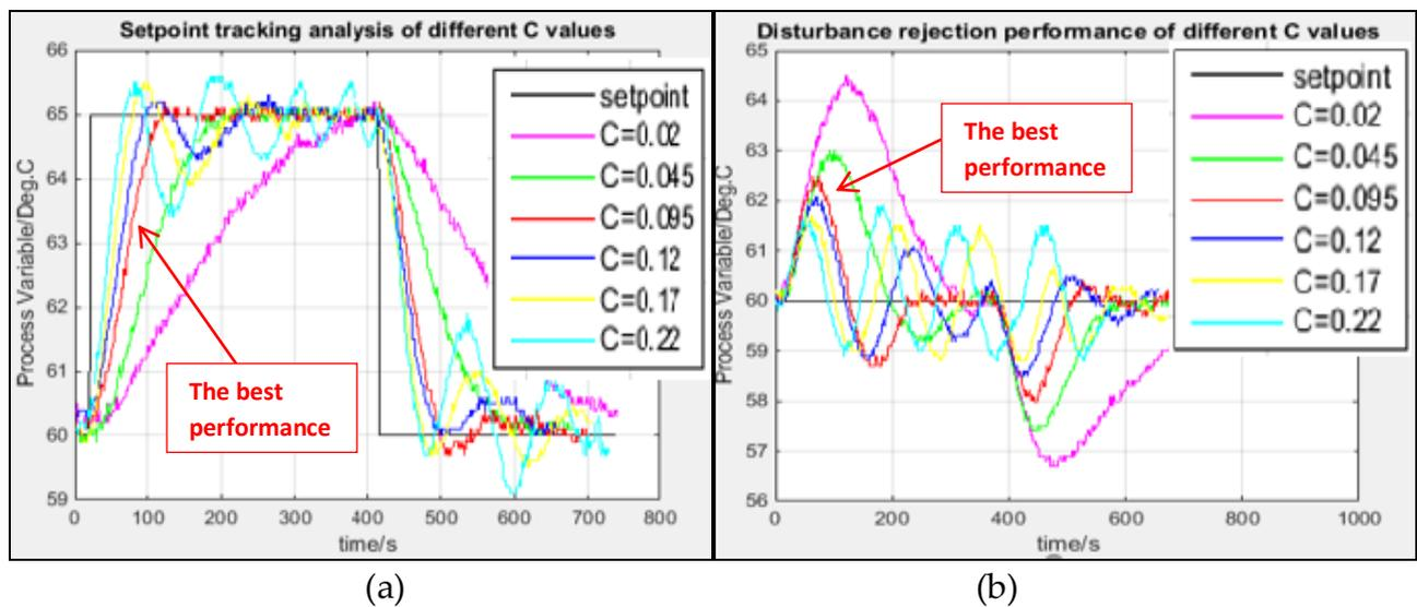
**Figure 5.** Servo and regulatory responses of various compensator ratios.
