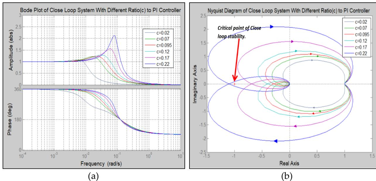
Figure 4. Bode diagram of various compensator ratio, *C*
