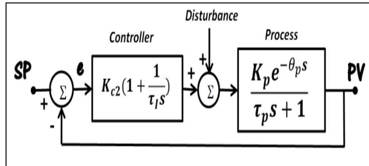
Figure 1. Block diagram of feedback control system.
