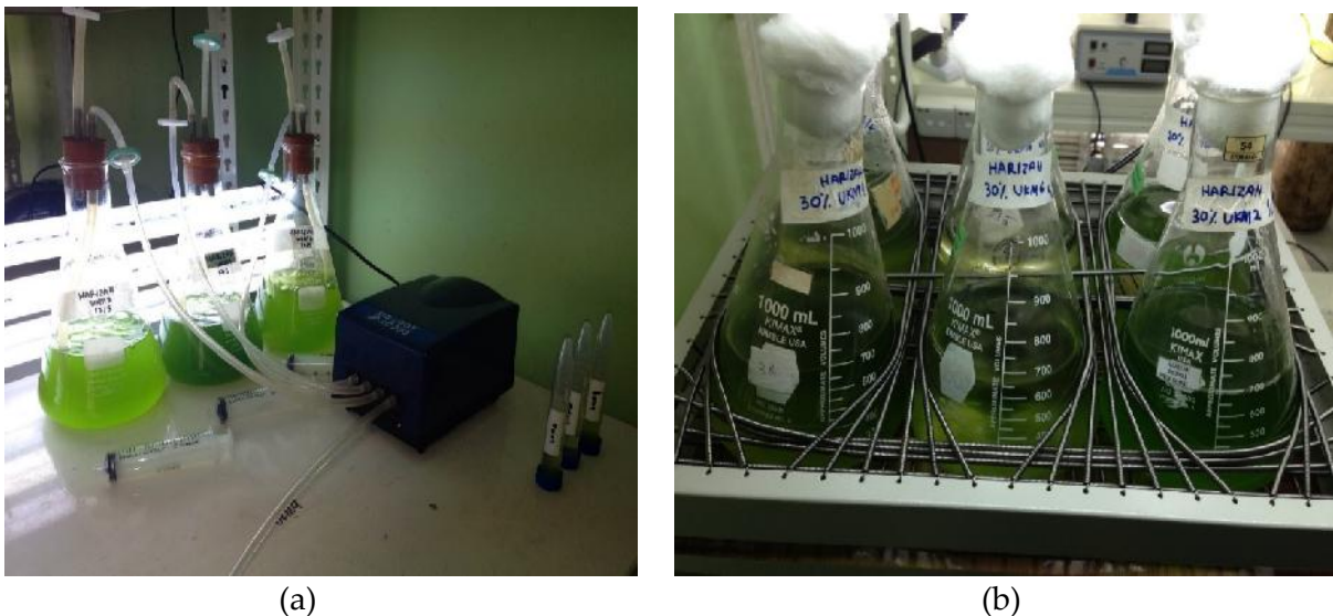
Figure 1. Experiment set up for microalgae cultivation in BBM a) Cultivation of microalgae with air supply from the air pump; b) Cultivation of microalgae with mixing by using shaker
