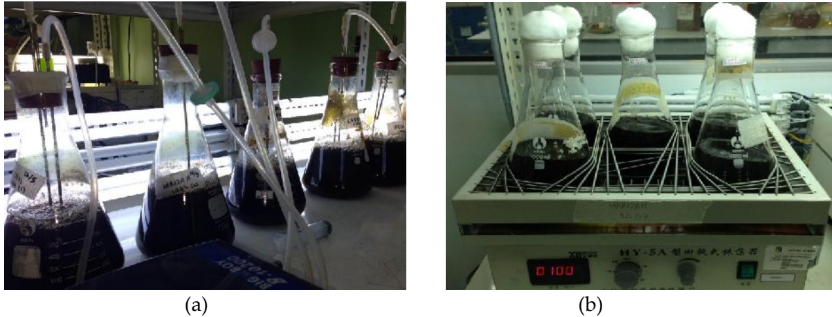
Figure 2. Experiment set up for microalgae cultivation in POME a) Cultivation of microalgae with air supply from the air pump; b) Cultivation of microalgae with mixing by using shaker
