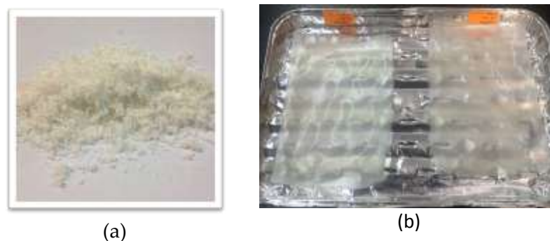
Figure 1. (a) The treated rice husk 700°C for 12 hour and (b) final composite of TPS/RHA after thermal treatment at 80°C for 24 hours.
