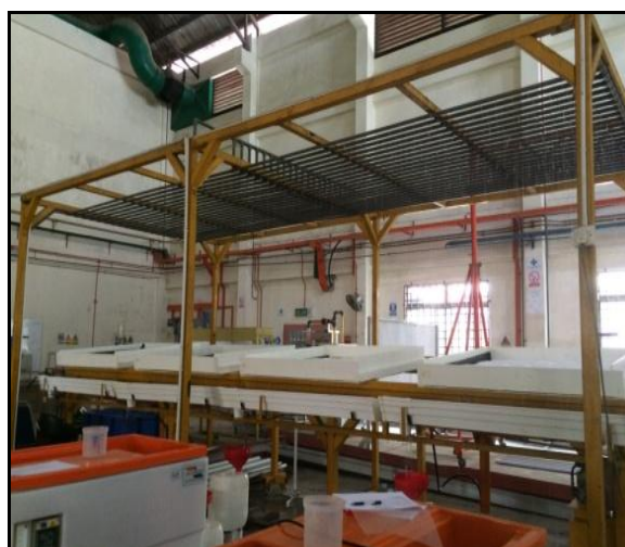
Figure 1. Testing under rainfall simulator (Asman et al., 2016).
