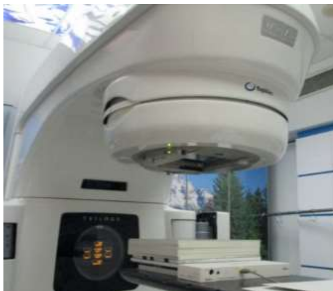
Figure 1. Varian Trilogy Clinac iX 10 MV photon beam (source: Tan Tock Seng Hospital (TTSH) Singapore)
