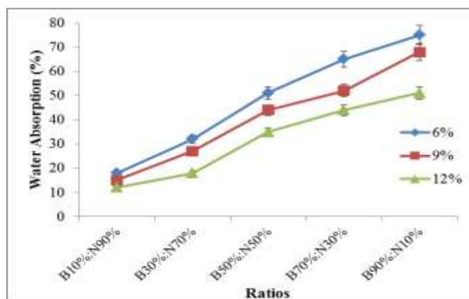
**Figure 3.** Percentage of water absorption of degradable bioplastic with 6%, 9% and 12% industrial cement.
