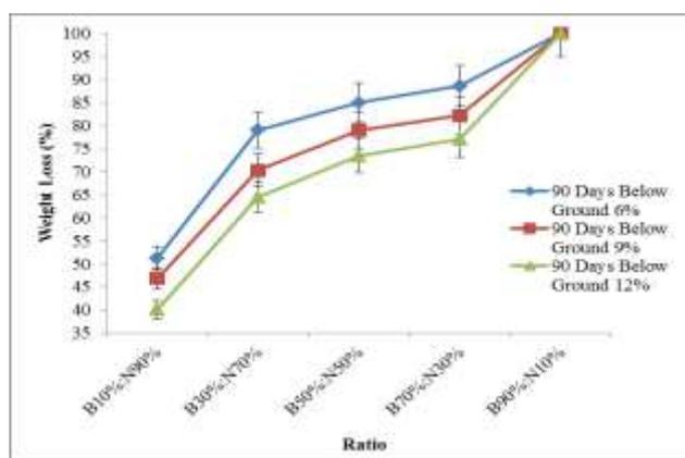
**Figure 2.** Weight loss percentage of degradable bioplastic pot with different ratios of bioplastic and different percentage of industrial cement that were tested below ground for 90 days.
