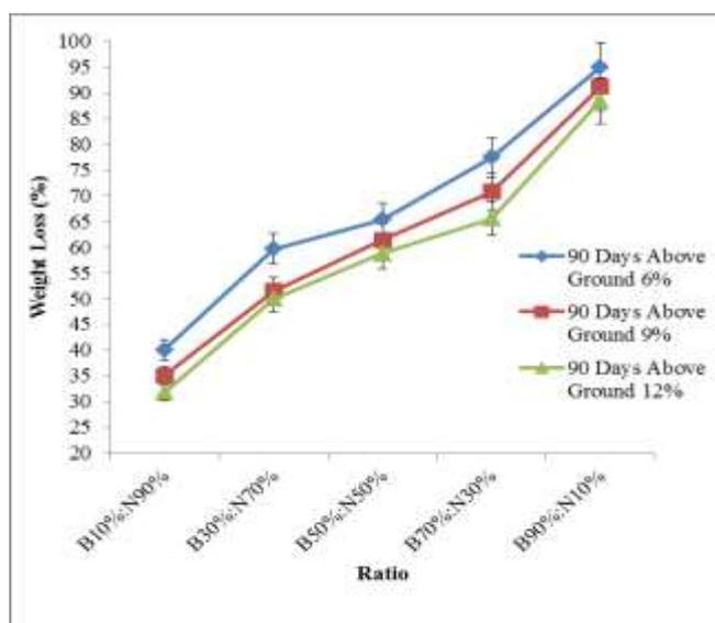
**Figure 1.** Weight loss percentage of degradable bioplastic pot with different ratios of bioplastic and different percentage of industrial cement that were tested above ground for 90 days.
