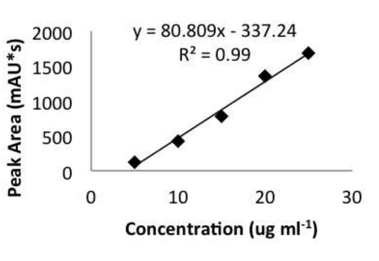
Figure 2: Calibration curve of quercetin standard
