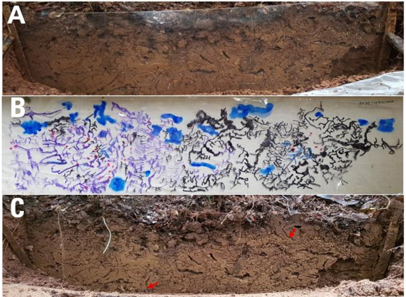
Figure 4. Plot results of an in-situ modified-rhizotron which includes photographs and a manual tracing of earthworm burrowing activity. (A) Measuring burrow length based on photograph using ImageJ software. (B) Tracing of burrows. (C) Visual assessment to verify manual on-site drawings.
