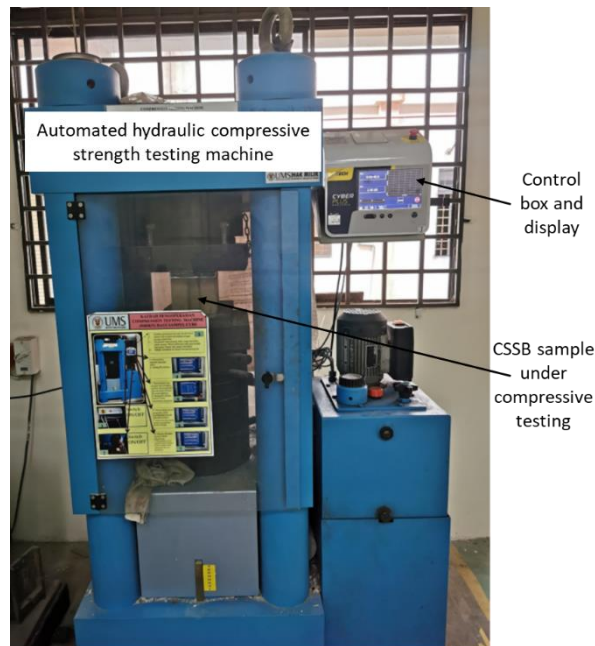
Figure 4. Compressive strength testing of CSSB sample
