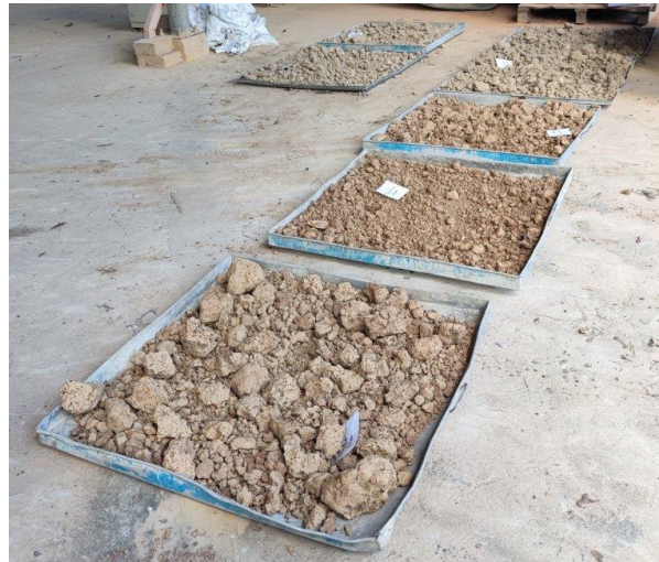
Figure 2. Open space drying of the sludge sample
