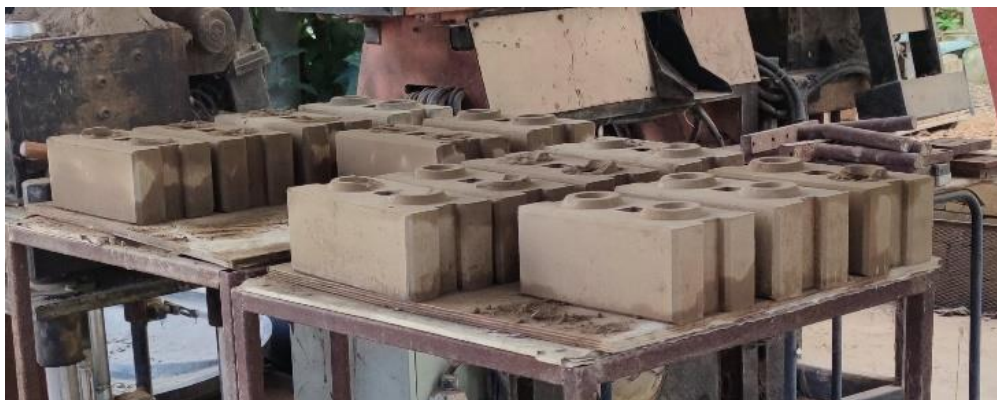
Figure 3. The finished interlocking CSSB bricks
