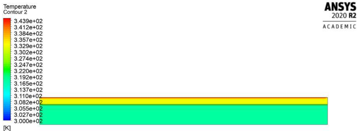
Figure 2. Temperature distribution at cross-sectional front view (normal to airflow direction) in CU-FL SHC.
