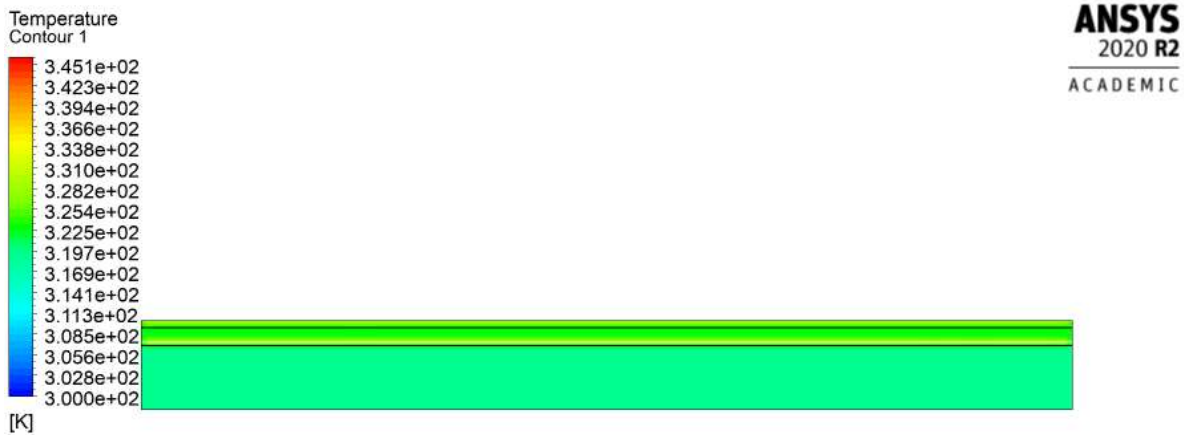
Figure 3. Temperature distribution at cross-sectional front view (normal to airflow direction) in CU-VG SHC.
