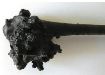
Figure 4. Solid carbon deposited on cathode (9 mm cathode diameter).
