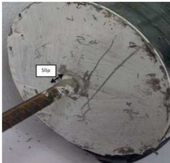
**Figure 5.** Reinforcement bar slip of pull-out failure
