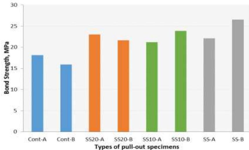
**Figure 6.** Bond strength of pull-out specimens
