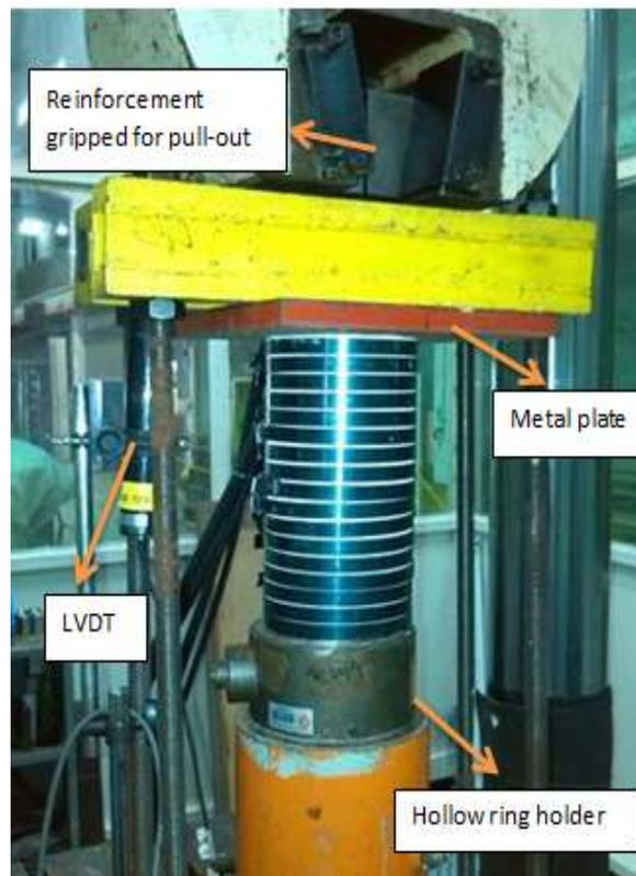
Figure 4. Specimen arrangement for pull-out test
