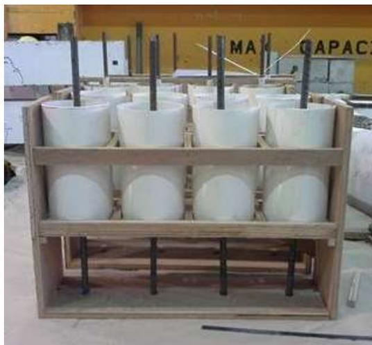
**Figure 2.** Pull-out test mould.
