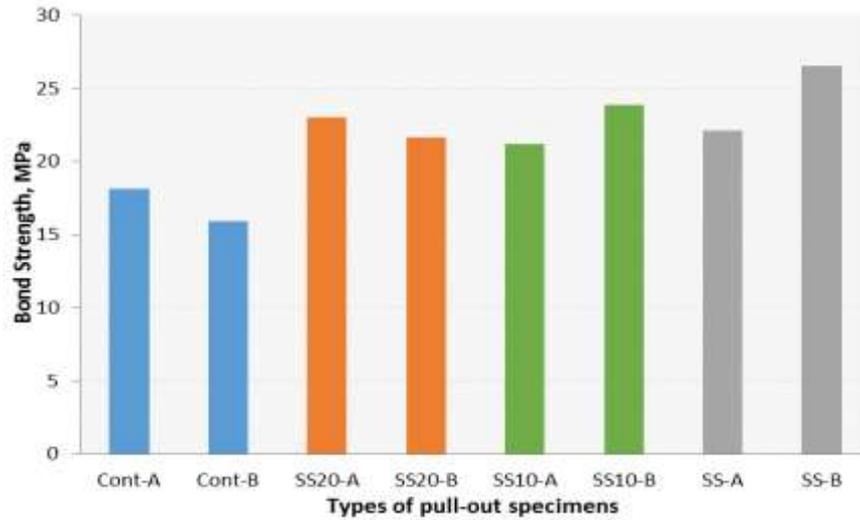
**Figure 6.** Bond strength of pull-out specimens
