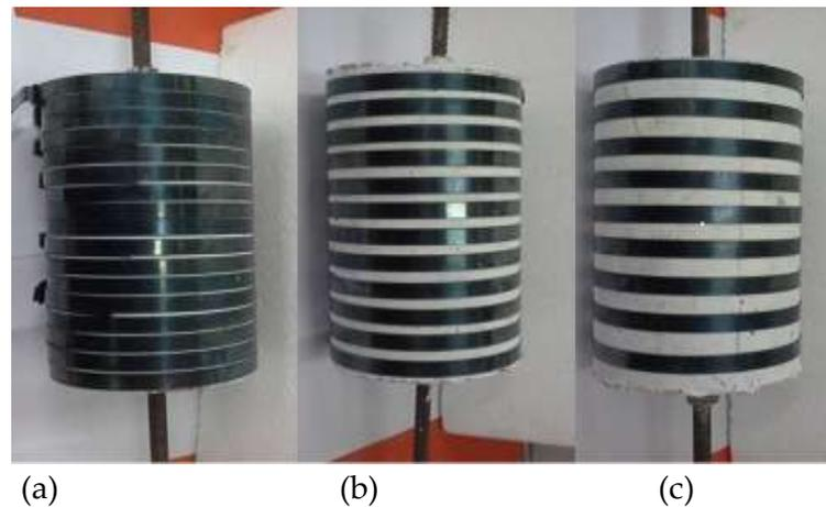
**Figure 3.** Pull-out specimens with: a) single layer steel strap with no spacing; b) single layer steel strap with 10mm spacing and c) single layer steel strap with 20mm spacing
