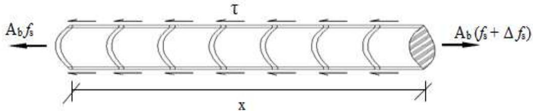
Figure 1. Equilibrium conditions of reinforcement due to external force.
