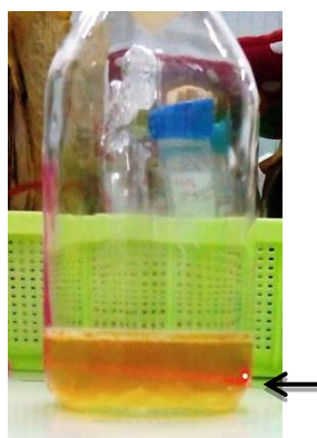
Figure 2. AgNp colloids synthesized by BAGBK-3. Red line appeared (arrowed) after exposed to laser beam
