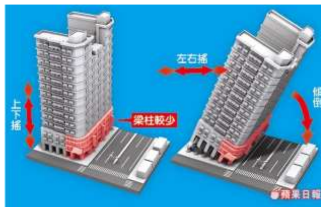
Figure 7. Schematic of Weiguang Building Collapse (Appledaily, 2016)
