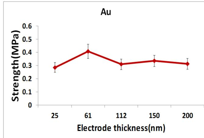
**Figure 2:** Adhesion test result of Au electrode
