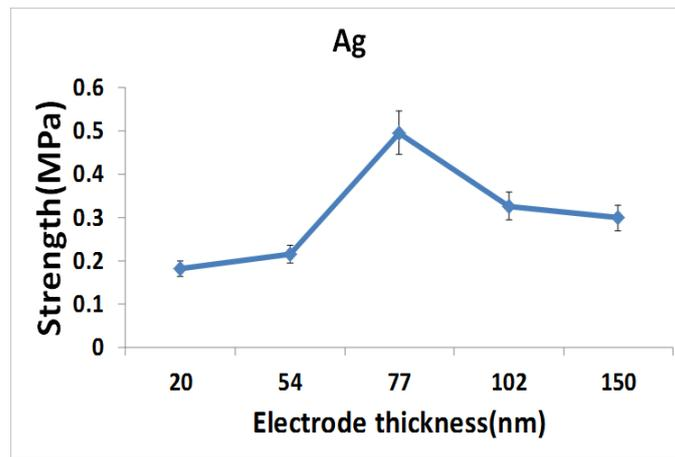
**Figure 4:** Adhesion test result of Ag electrode
