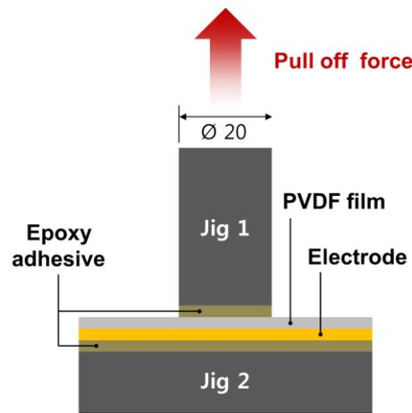
**Figure 1:** Schematic configuration of adhesion tests
