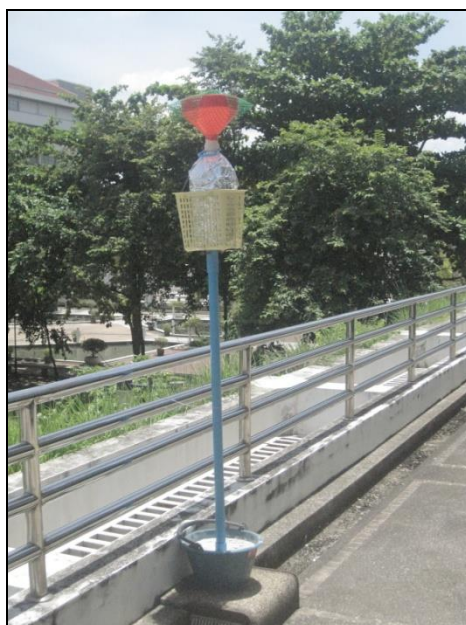
Figure 2: The dust fall sampling equipment
