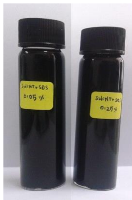
Figure 2: SWCNT nanofluids after 1 month.
